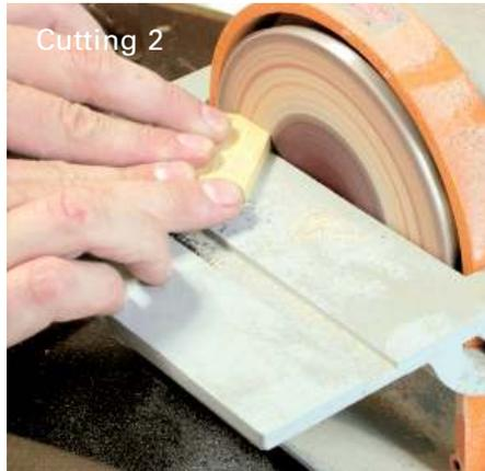
A belt sander, drill or grinder equipped with a sanding disc can also be used to quickly shape tiles.
